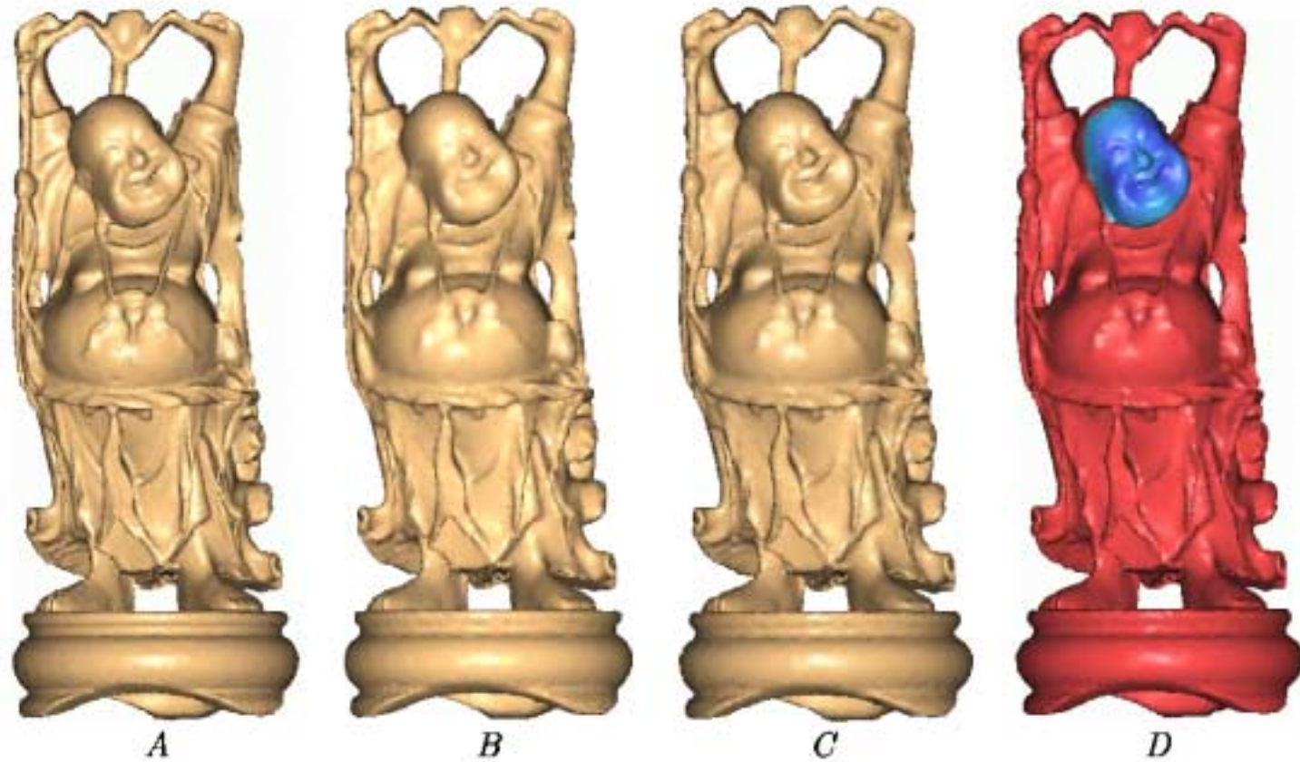
Figure 24: A: Buddha model of 334 K triangles. B: simplification with 46 K triangles using a uniform tolerance. C: simplification with 49 K triangles using a variable tolerance. D: coloring of the tolerance volume for the surface of C, with increasing values from blue to red in a Rainbow colormap.
