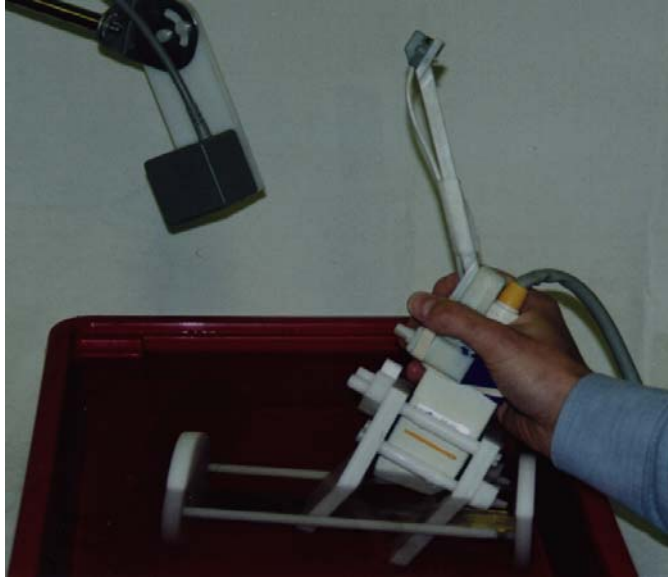
Figure 6: Calibration using the Cambridge phantom. A 7 MHz linear phased array probe is fitted into the phantom's clamp, which itself is fitted around the brass bar immersed in the water bath. The position sensor's transmitter is suspended from a cantilevered support above the water bath, while the receiver is attached to the probe at the end of a rigid mount.
