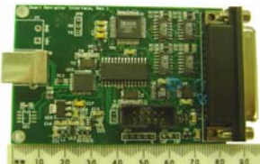
Figure 3. Retractor oxygenation sensor interface circuit board
