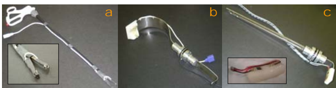
Figure 4. Sample sensing retractors: a) laparoscopic Babcock grasper, b) Deaver retractor with force and oxygen sensing and c) customized Balfour retractor with force and oxygenation sensing
